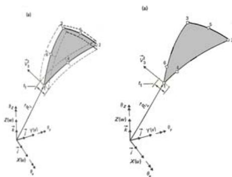
Fig. 2(a) Iso-parametric triangular shell element TRIA6 (b) Singular Iso-parametric triangular shell element STRIA6
