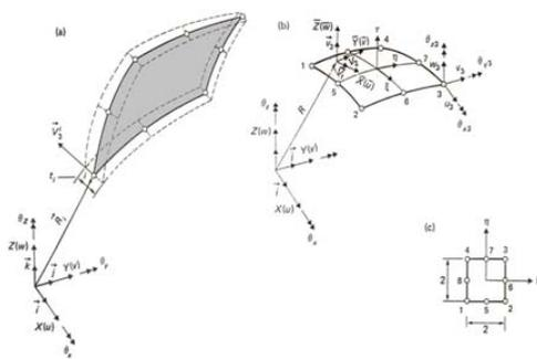
Fig. 1 Iso-parametric quadrilateral shell element QUAD8
