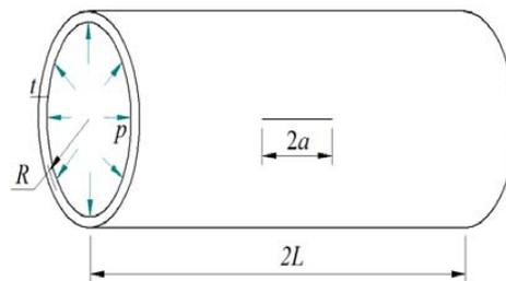
Fig. 3: Pressure loaded cylinder with axial crack
