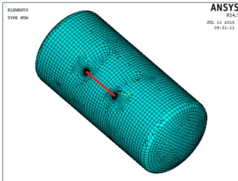
Fig 6 FE Model of Axial Crack in cylindrical region
