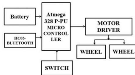
Figure. 2 Vehicle Hardware Unit
