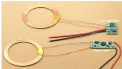
Figure. 3 Transmitter and Receiver Unit
