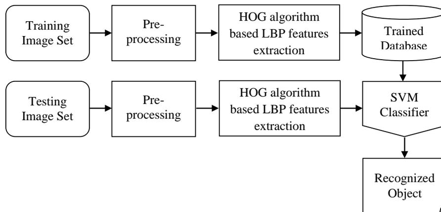
**Figure 1 HOG Algorithm Based Object Recognition System**
