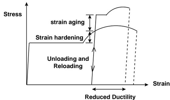
Figure. 4 Effect of Cold Working on Steel Behaviour
