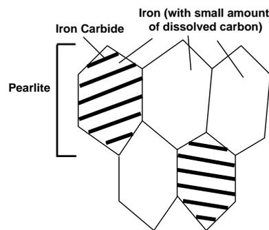
Figure. 1 Microstructure of Normalised Steel
