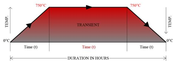
Figure. 9 Steel beam under temperature upto 750°C
