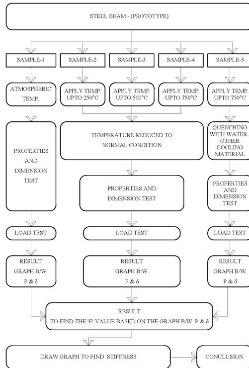
Figure. 5 Methodology flow diagram
