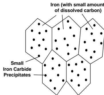
Figure. 3 Microstructure of Quenched and Tempered Steel
