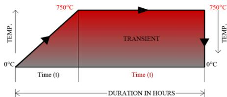
Figure. 10 Steel beam under temperature upto 750°C & quenching
