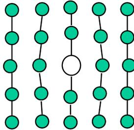
Figure. 2 Distortion of Crystal Lattice due to Mismatch in Atomic Size
