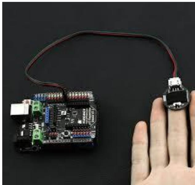
through that organ (a vascular region). In case of applications where heart pulse rate is to be monitored, the timing of the pulses is more important. The flow of blood volume is decided by the rate of heart pulses and since light is absorbed by blood, the signal pulses are equivalent to the heart beat pulses.
