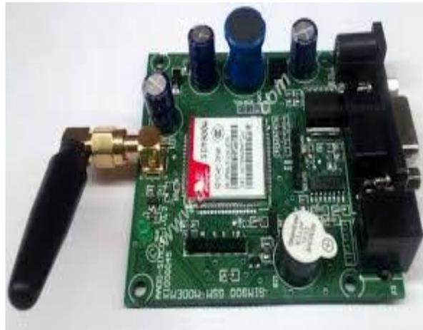
connection. A GSM modem can also be a standard GSM mobile phone with the appropriate cable and software driver to connect to a serial port or USB port on your computer. GSM modem is usually preferable to a GSM mobile phone. The GSM modem has wide range of applications in transaction terminals, supply chain management, security applications, weather stations and GPRS mode remote data logging.
