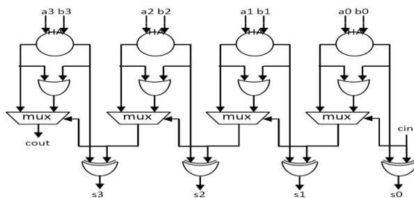
**Fig 1.Circuit diagram for 4-bit EHRCA circuit**
