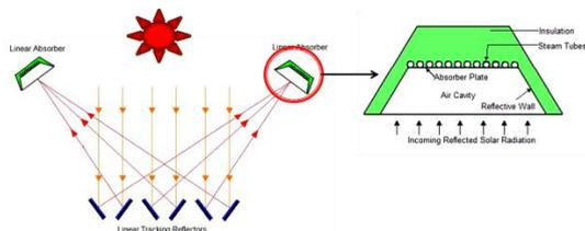
FIGURE 3. Linear Fresnel reflector
