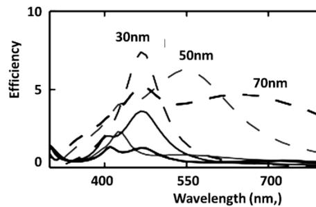
FIGURE 10. efficiency profile of absorption (solid) and scattering (dashed) using PSC with cross sections of sphere radii of 30nm, 50nm and 70nm.
