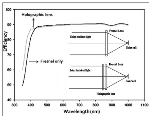
FIGURE 9. Efficiency profile of optical concentrator using Fresnel lens only (black) and Holographic lens (gray) tends to gain on 2%.
