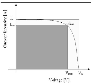
FIGURE 2. Tracing IV-solar cell Curve used in the design of the new concentrators, measured under standard conditions. The measurement was performed on a 123 mm x 125 mm cell.
