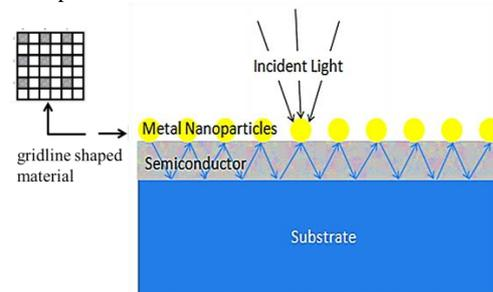
FIGURE 8. Plasmonic Solar Concentrator (PSC) using metal nanoparticles
