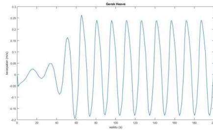
**Fig. 6.** Simulation result for heave velocity without controller
