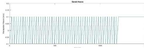
**Fig. 7.** Simulation result for heave velocity using NMPC
