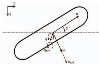
**Fig. 4.** BFF and EFF coordinates in longitudinal model [1]
