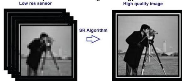
Fig 2. Concept of super resolution (from LR images to HR image)
