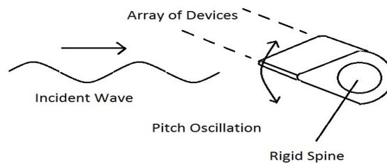
(Fig-3.4.1 Wave Action on Salter Duck Structure)
