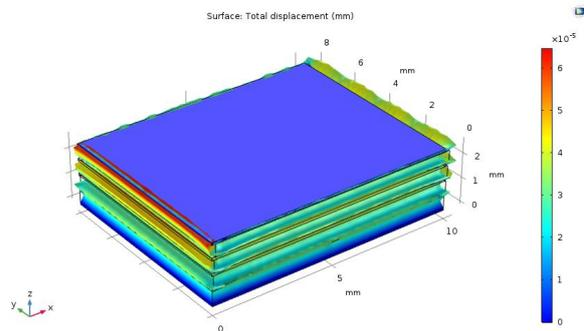
Figure 4 Displacement of Multi step piezoelectric actuator at 100V
