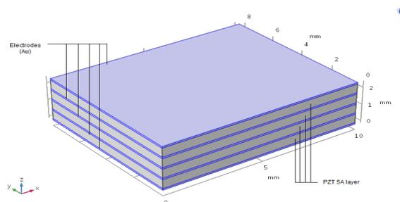
Figure 1 Multilayered Piezoelectric actuator model
