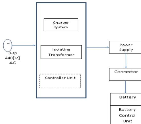
Fig. 1. Charger System of Battery Schematic Diagram
