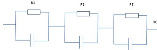
Fig. 2 Circuit Model of SAFT
