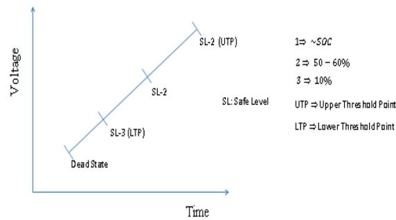
Fig. 4. Safe Level of Battery System
