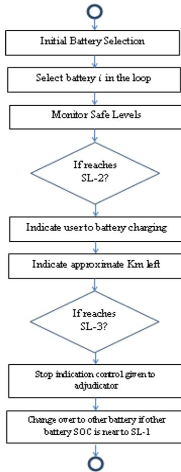
Fig. 5. Flowchart for Battery Management Model
