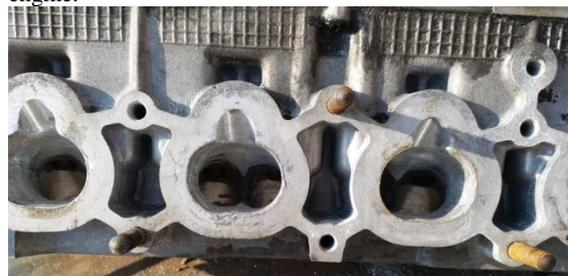
Fig. 10 Well-Ported and Polished Race Engine Intake
