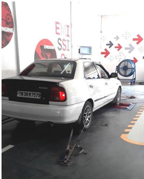
Fig. 8. Dynamometer Testing of Maruthi Baleno Vehicle
