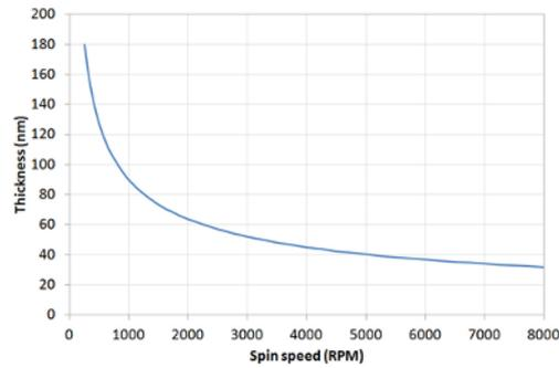
Figure 3. Thickness vs. speed graph
