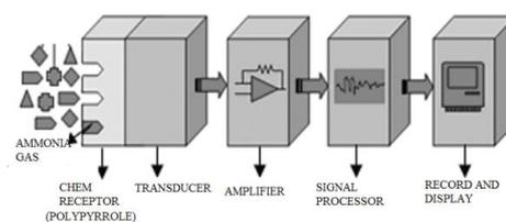
Figure 1. Block diagram with chem-sensor
