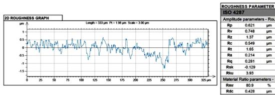
Fig. 8. 2D Roughness profile of uncoated piston ring
