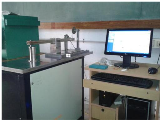
Fig. 3. Pin On Disc Tribometer (Wear & Friction Test)
