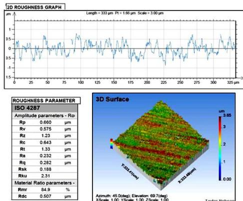
Fig. 10. 2D Roughness Profile of Al<sub>2</sub>O<sub>3</sub> coated piston ring
