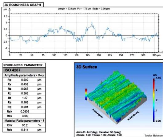
Fig. 9. 2D Roughness Profile of TiO<sub>2</sub> coated piston rings
