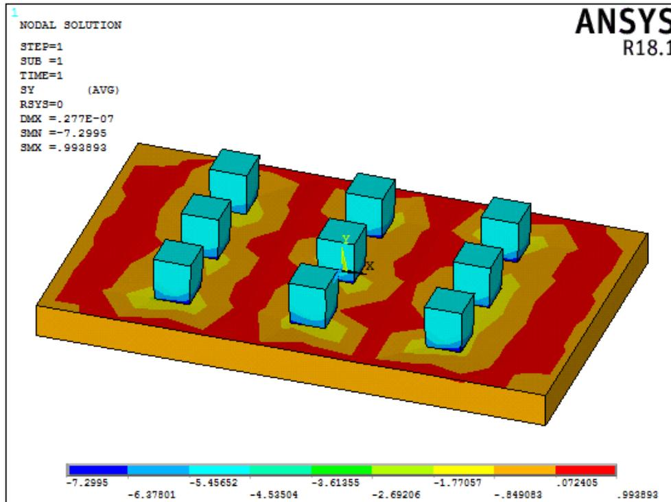
Figure 2 – Analysis result from ANSYS for mild steel
