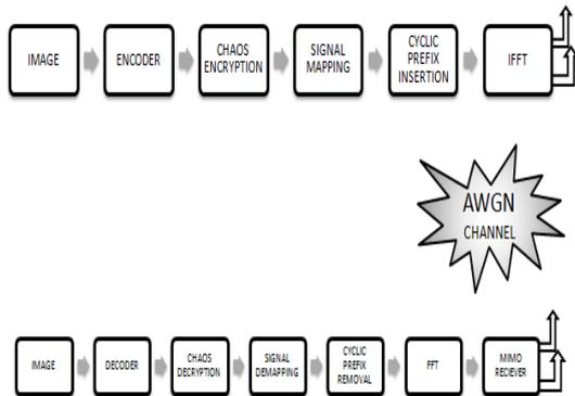
Fig. 4: Block Diagram Of This Concept
