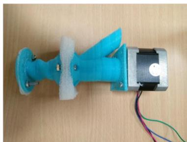
Fig. 3. Fully assembled Progressive cavity pump setup
